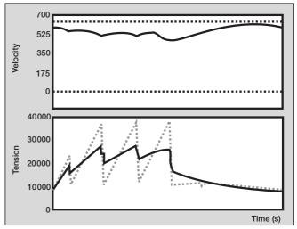
Fig. 10: Belt velocity and belt tension vs. time at an intermediate drive
