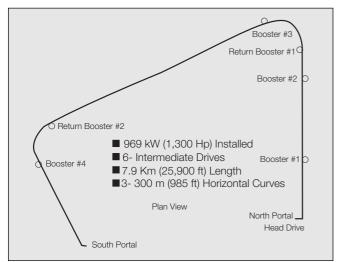
Fig. 15: Intermediate drives configuration of the conveyor contructed for the tunneling project at the Yucca Mountain Nevada Nuclear Waste Depository
