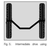
Intermediate drive using tires to transmitt the power
