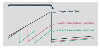
Fig. 3: Belt tension diagramm
