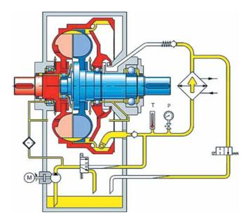
Fig. 9: Voith TPKL variable fill fluid coupling
