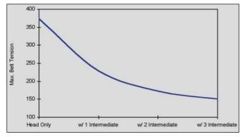
Fig. 4: Maximum belt tension vs. number of drives
